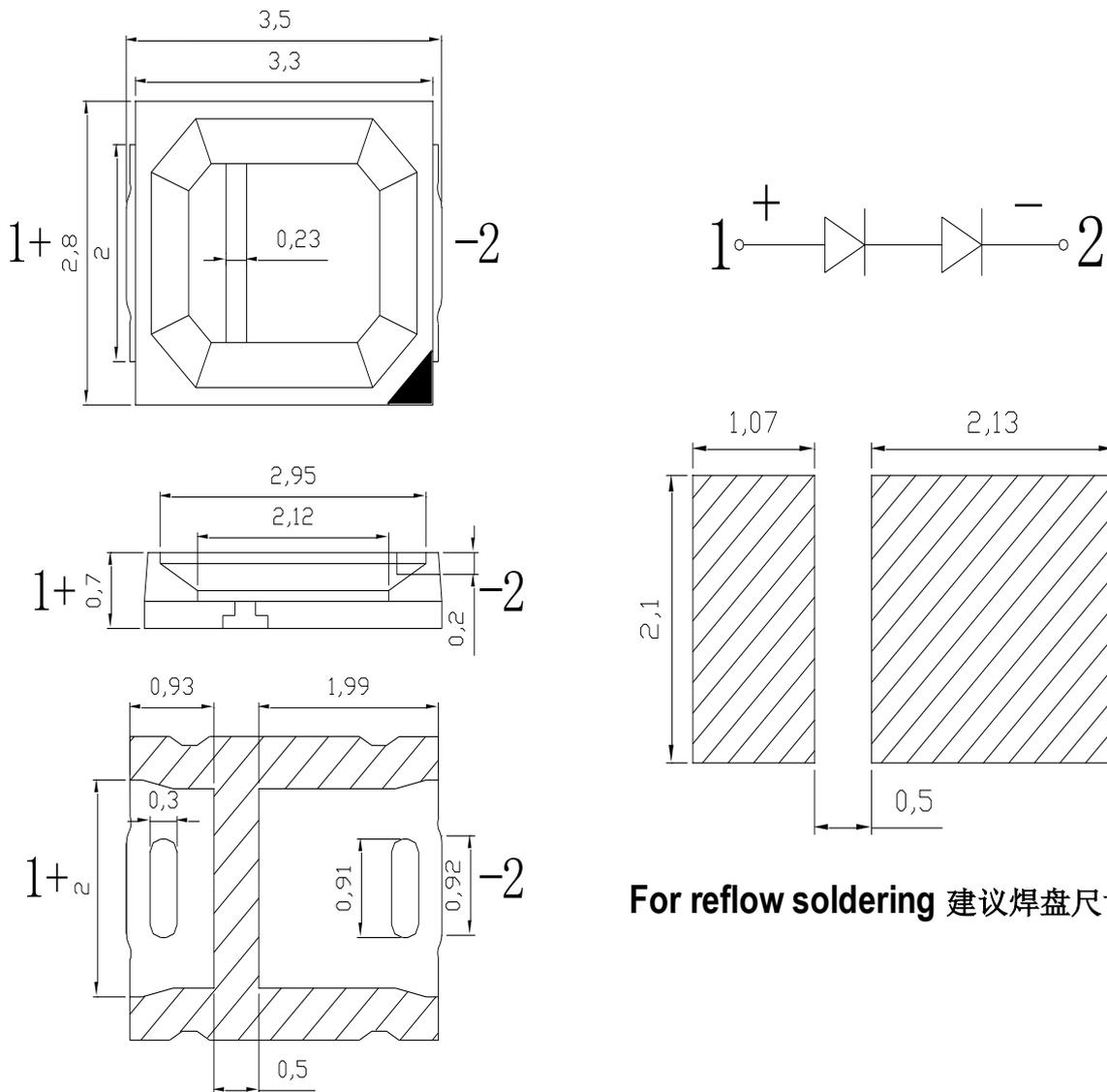
For reflow soldering 建议焊盘尺寸
